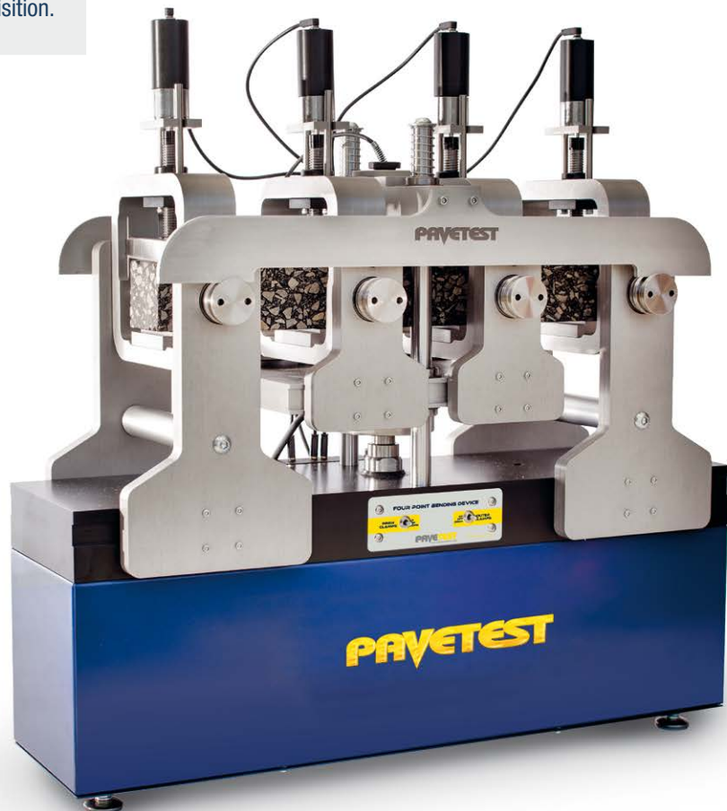
B210-01 Servo-pneumatic four point apparatus
