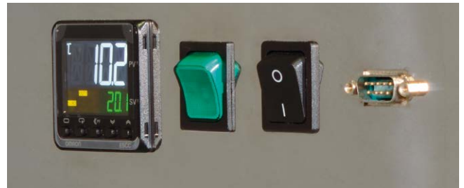
Cabinet switches and temperature controllers
