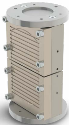
B204 KIT Overlay kit according to ASTM WK26816
