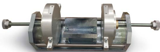
B282-08 TSRST specimen gluing jig (needed accessory)
