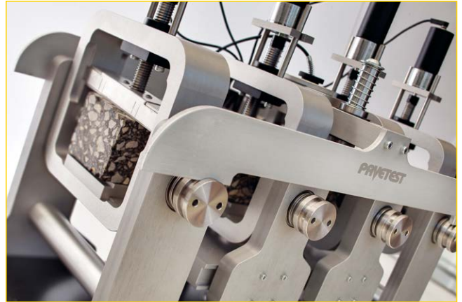
B210-01 Servo-pneumatic four point apparatus, detail
